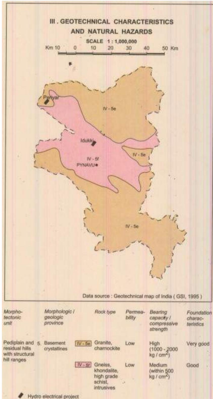
Figure 4: Geotechnical characteristics and natural hazards map of Idukki. (Source:
